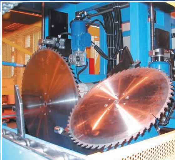
The Easy-Cut 4 Saw is a power-assisted, manually set up component saw, where all axis positions are set up using push-button control and LCD read-outs at two control panels.
