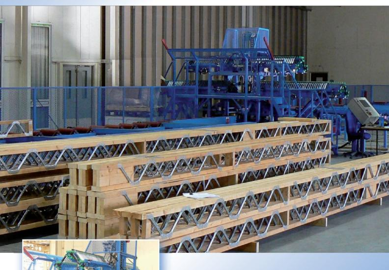
The ReVolution has a unique and patented vertical pressing station with CNC controlled positioning of the Posi-Strut<sup>™</sup> webs ensuring precise and accurate placement every time and eliminating lengthy setting up procedures. Capable of over 1500m in a single shift.
