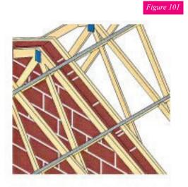
The Building Designer should ensure that, when required, adequate holding down fixings, 'C', are specified for both the trussed rafter and the wall plates or bearings.
