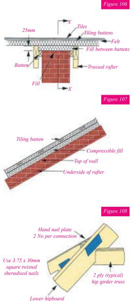
Hipboard to be notched over girder truss and butted together over centre of girder.
