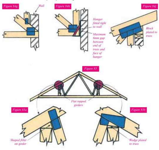
Top hung fixings (figure 84j) are not common since, at ceiling level, the wall generally needs lateral restraint from the roof against wind and the ceiling ties need to be stabilised. Flat topped girders supporting trusses (figure 85) can be supplied with a shaped fillet (figure 85a); or trusses may have a wedge or block plated into the joint to provide a horizontal bearing surface (figure 85b).
