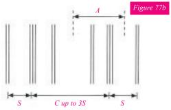
When the two trimming trusses at each side of the opening (figure 77b) are actually nominally fixed together with nails, at say 600mm centres along all members, an opening of up to three standard spacings may be used. Deeper purlins, binders and ridge board of typically  $47 \times 175$ mm and trimmers of  $47 \times 125$ mm should be installed.
