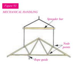
Where bundles of trusses are raised to roof level, caution should be exercised in the removal of the restraining bands (see section 3.11 figure 92). Should these bundles of trusses be stored either on a temporary working platform or at eaves level, the contractor should take the necessary steps to ensure that the supporting structure has sufficient strength and that a storage system as illustrated in either figure 90 or 91 is constructed.
