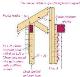
Purlin support post. Size 50 x (W + 25), extending to ceiling joist. Fix with one row of 4.0 x 100mm long round wire galvanised nails at 80mm centres for full length of post
