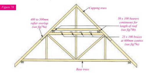
The two tier truss (figure 78) comprises a flat-topped base truss and a triangular capping truss, fitting alongside the base truss on longitudinal bearers. Each truss may be one of a large selection of types. The base truss will generally be made as high as practical but not so high that the span of the capping truss is less than 2-3m. Although a duo-pitched shape is shown in figure 78, all basic configurations can be constructed by the two tier method.
