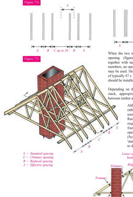
Figure 77a shows a system suitable for openings greater than 10% over standard and up to twice standard spacing. Battens and plasterboard should be given extra support.
