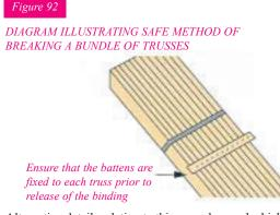
Alternative details relating to this procedure and which involve the unbundling of the trusses whilst on the back of the lorry should be communicated by the contractor to the truss manufacturer prior to their delivery to site.
