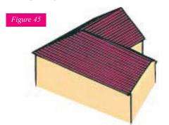
Hipped corners for mono-pitched and other roof shapes are based on the same principles described below for duo-pitched roofs.
