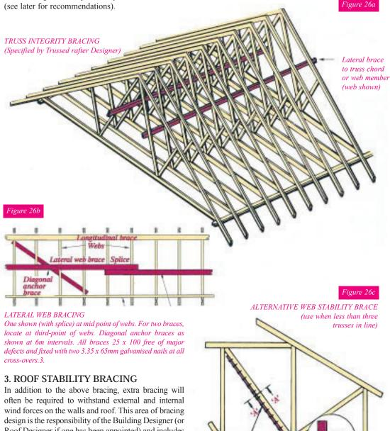
design is the responsibility of the Building Designer (or Roof Designer if one has been appointed) and includes such areas as diagonal wind bracing, chevron bracing to internal members, longitudinal bracing at truss node points, etc.
