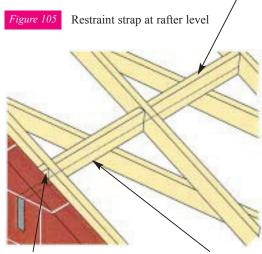
Packing piece between inner leaf and first rafter Strap bedded under a cut block
