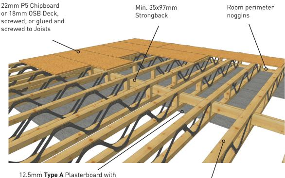
12.5mm **Type A** Plasterboard with 5mm skim. Drywall screws at 150mm centres
