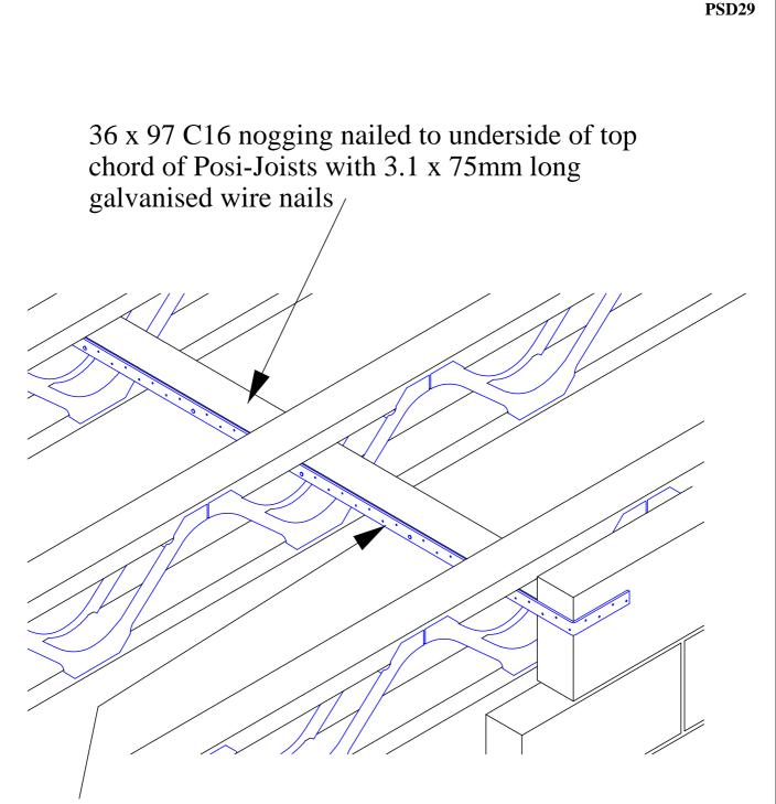
Strap fixed to nogging with a minimum of four fixings of which, at least one is to be over the third joist.
