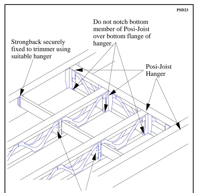
Twice nail brace to web using 3.1 x 75mm long galvanised wire nails
