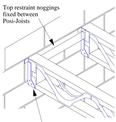
Do not notch bottom member of Posi-Joist over bottom flange of hanger.
