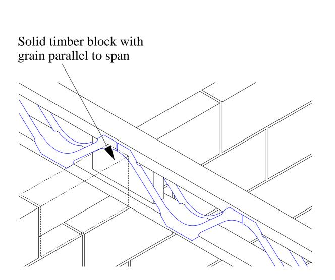
Note: Use on internal load bearing internal walls (not fire walls). Full blockfill only required when there is a load bearing wall above the floor level
