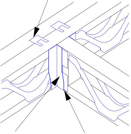
Posi-Joist Hanger Do not notch bottom member of Posi-Joist over bottom flange of hanger.
