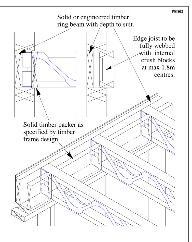
Bottom Chord Support Timber Frame External (With Ring Beam And Packer)
