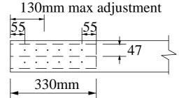
Block nailed to top and bottom chords using 6 No. 3.1mm diameter 90mm long power driven annular ring-shank nails at 44mm centres.
