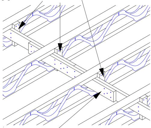
1200mm long splice fixed with 10 no 3.1x 75mm galvanised wire nails each side of splice, nailed through and clenched over on far side
