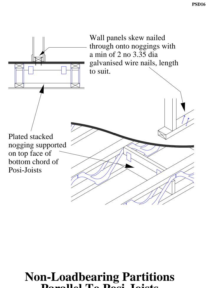
Parallel To Posi-Joists (Alternative Nogging Support Detail)
