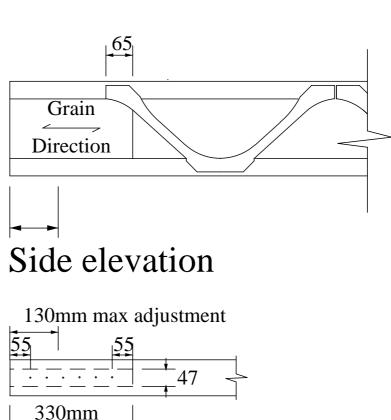
Block nailed to top and bottom chords using 6 No. 3.1mm diameter 90mm long power driven annular ring-shank nails at 44mm centres.
