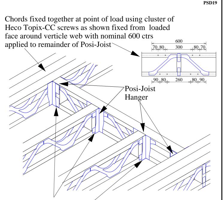
Do not notch bottom member of Posi-Joist over bottom flange of hanger.
