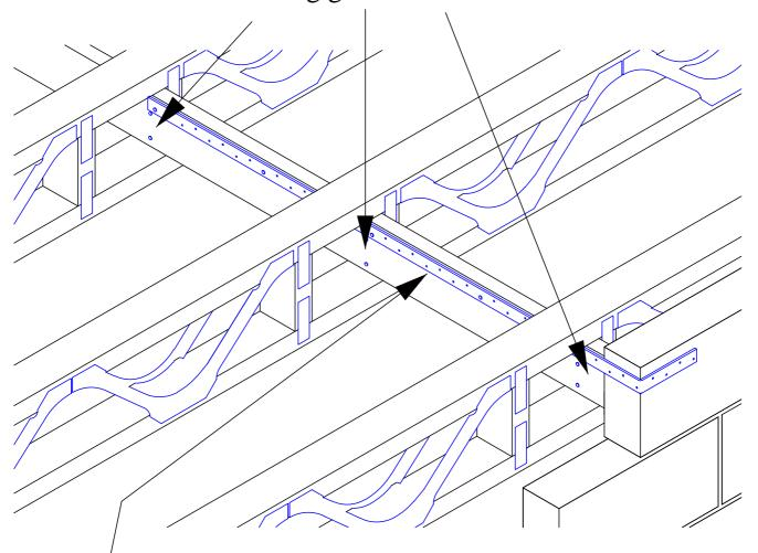
Strap fixed along top edge of strongback with a minimum of four fixings of which at least one is to be over the third joist.
