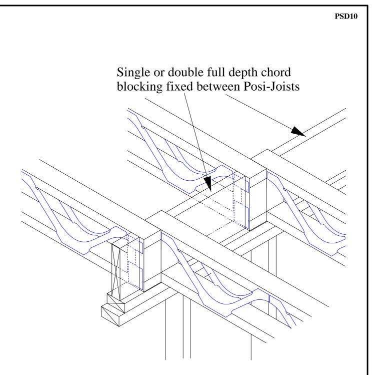
Bottom Chord Support Timber Frame Internal Lapped (With Full Depth Strutting)
