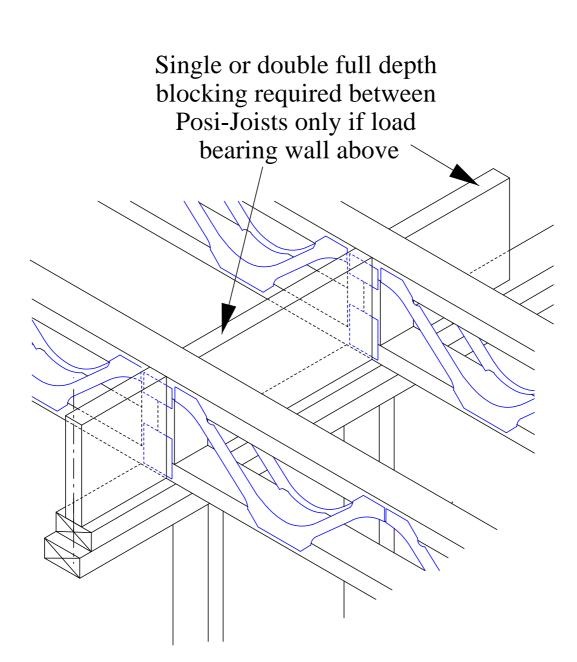
Bottom Chord Support Timber Frame Internal Continuous (With Full Depth Strutting If Required)
