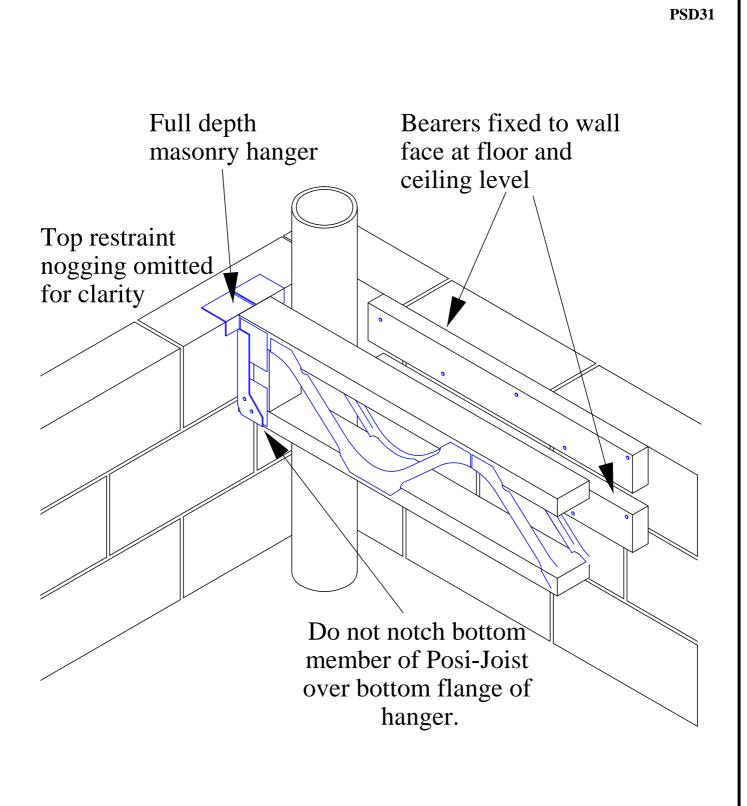
This may not perform well acoustically as sound will be transmitted directly from the floor to the bearer through the inner leaf of the wall.
